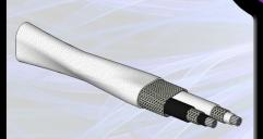
Two high purity silver plated copper conductors surrounded by individual silver plated copper braided shields. Each conductor is fabricated using 19 very fine individual wires wrapped in a low dielectric PTFE insulator. Conductors are shielded by a 75% minimum coverage silver plated copper braided shield. Manufactured and hand terminated in the USA.
